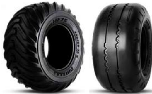
Figure 2. Tractive tread tire (left) and Smooth tread tire (right) [9]
