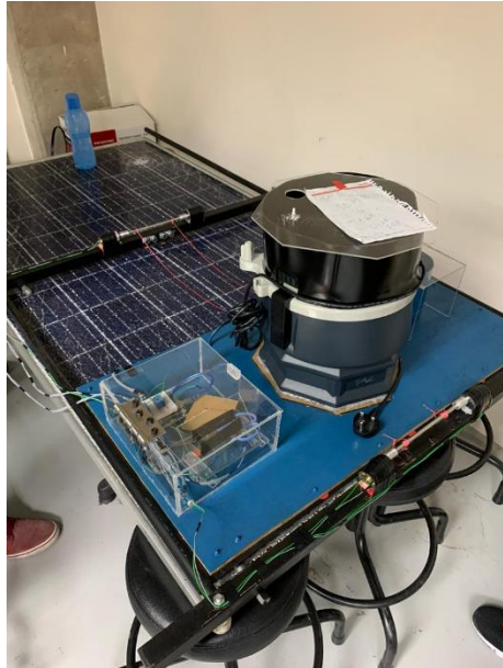
Figure 17: How to mount the prototype on the panel
