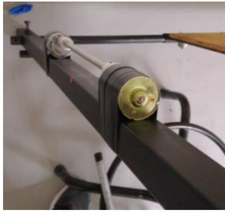
Figure 11: 2 Gear Motors making up one side of the winch mechanism
