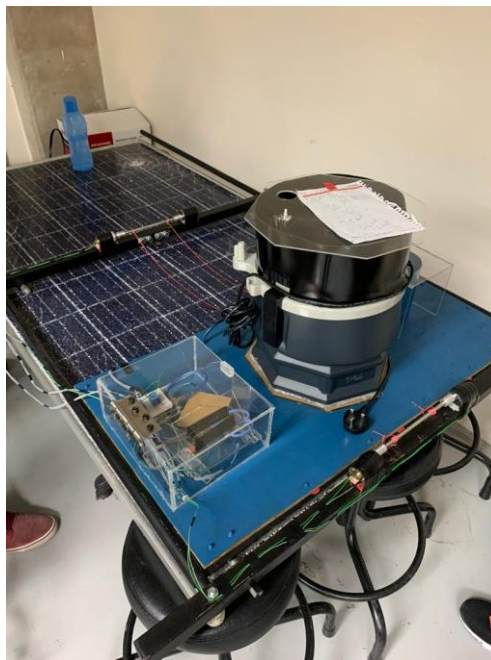
Figure 26: Team Solar Fam's Autonomous Solar Panel Cleaning Robot
