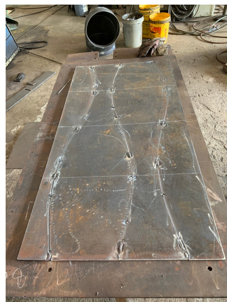
Figure 4.2 Subsections welded into piece of flat plate
