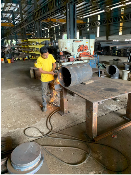
Figure 4.5 Cutting of the welded rolled plate
