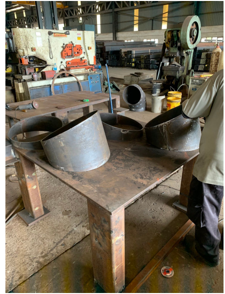
Figure 4.6 The subsections of the rolled plate
