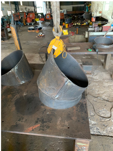
Figure 4.7 Joining of subsections
