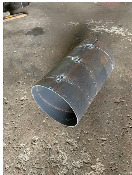
Figure 4.4 Welded plate after rolling
