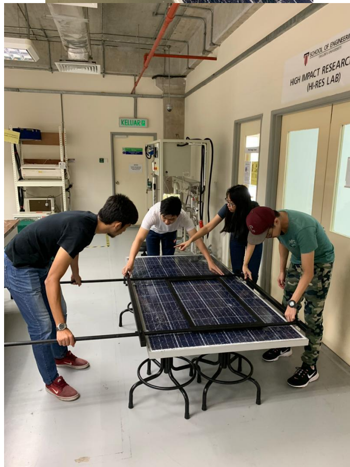
Figure 45: Testing the movement of the frame on solar panel
