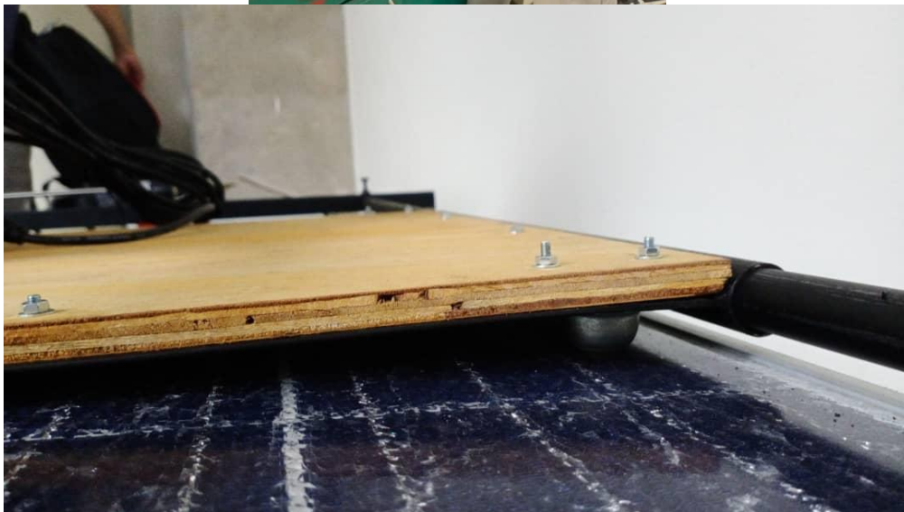
Figure 48: Securing wheel bearings underneath the wooden platform
