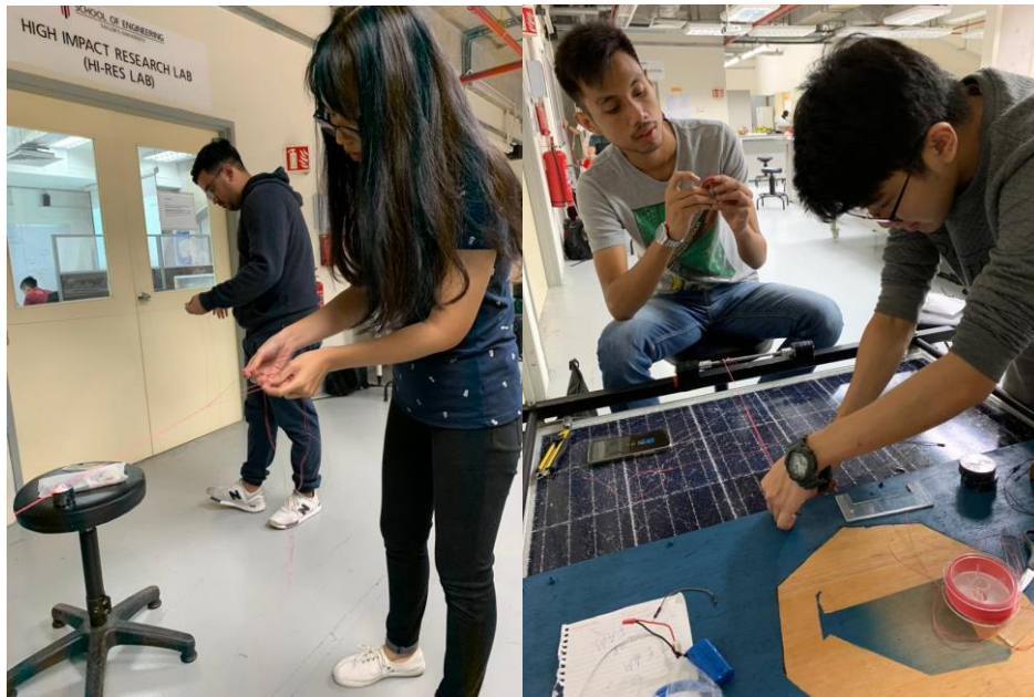
Figure 53: Braiding string to avoid tangling (left) and tying to platform and shaft (right)
